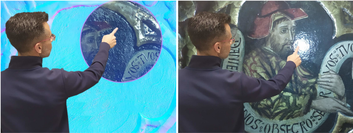
Fig. 25. Exploration of a painting (panel of the polyptych retable of Saint Bernardino (1455), Cagliari, Italy). The user explores the dataset using visualization lenses and relighting on a large multitouch screen. Left: the outside of the lens shows the normal map, while the inside shows a relighting from SV-BRDF. Right: the user interactively controls a spot light to relight the painting.
